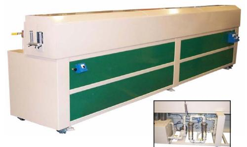
20' Cooling Tank with spray headers. Air operated lids. Double wall stainless and insulated.
