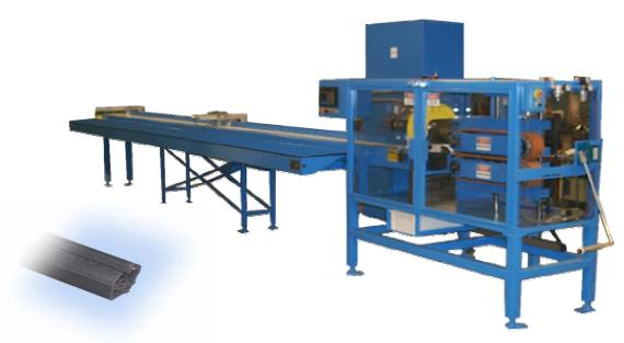
Online Extrusion Saw features servo control for high speed precision feed and cutting accuracy. Servo controlled cutting offers clean square cuts. Extended conveyor offers wide range of cutting lengths and side discharge of cut parts.
