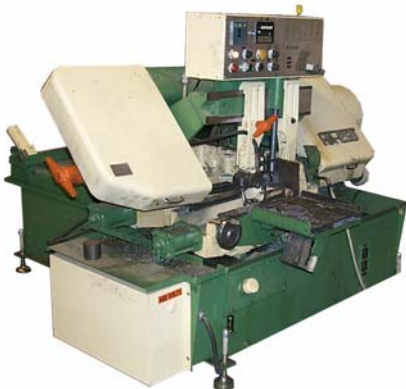
Automatic Sawing 8" Diameter 6x8 Capacity Length control +/-0.005
